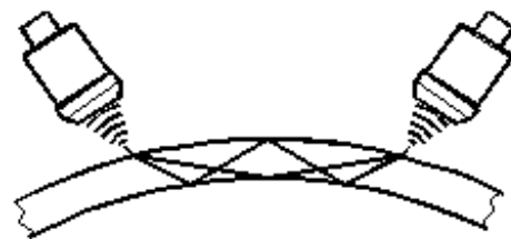
Figure 3 : Generation of plate waves
