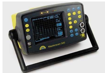
Figure 7 Sonatest MS340 Flaw Detector
