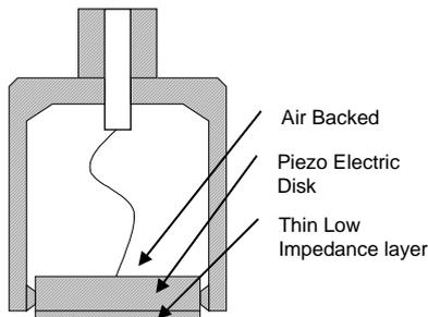
Figure 4 : Air-coupled probe design features
