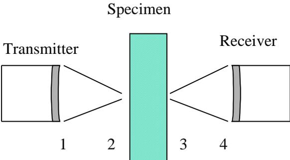
**Figure 3: Acoustic interfaces**
