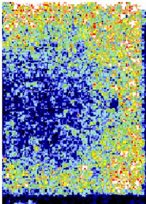
**Figure 11: C-scan image of a 15 x 20 cm.. section of a SiC panel scanned with 400 kHz air-coupled transducers.**
