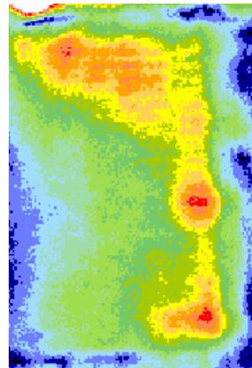
**Figure 12: C-scan image of a 15 x 20 cm.. section of a SiC panel scanned with 50 kHz air-coupled transducers.**
