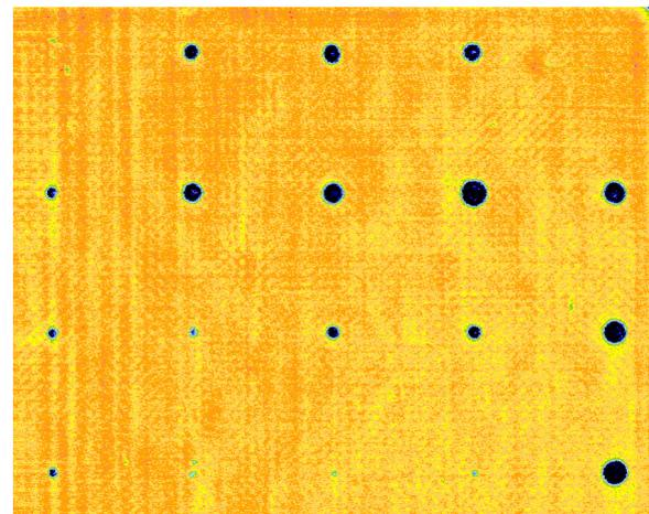
Figure 8: C-scan image with 400 kHz air-coupled transducers. The smallest resolved Teflon inserts in the bottom row measure 1.6mm. in diameter.
