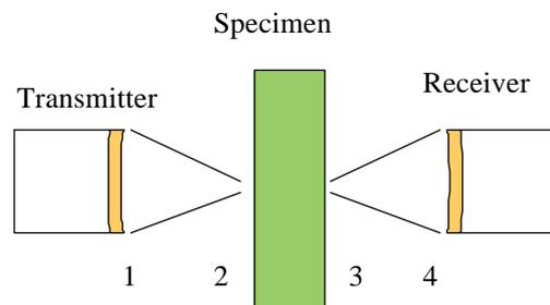
Figure 1: Losses at interfaces with Air-coupled UT
