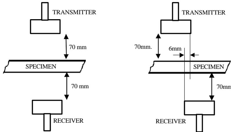
Figure 6: 50 kHz transducers:
