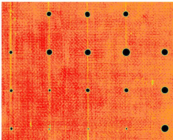
Figure 7: C-scan image with water squirters at 2.25 MHz. Teflon inserts measuring 1.6mm to 20mm at 100mm. Distances.
