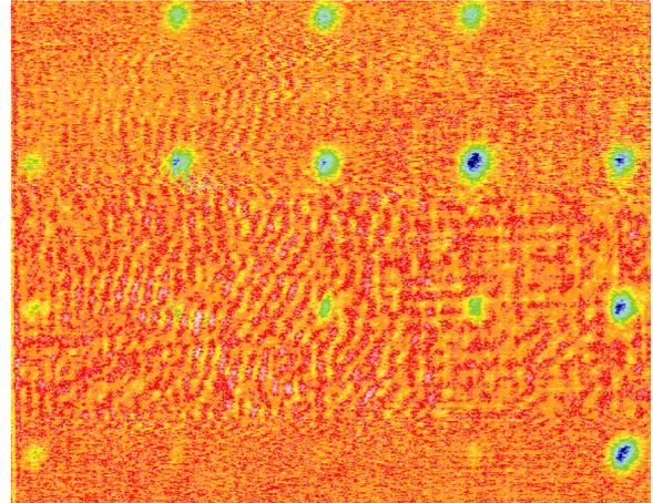
**Figure 10: C-scan image with 50 kHz transducers, laterally displaced, in through-transmission. Teflon inserts with diameters less than 8 mm. cannot be resolved.**
