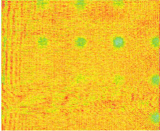
**Figure 9: C-scan image with 50 kHz transducers in straight through-transmission. Teflon inserts with diameters less than 12 mm. cannot be resolved.**
